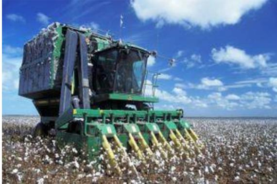
A [cotton picker](#) at work. The first successful models were introduced in the mid-1940s and each could do the work of 50 hand pickers.
